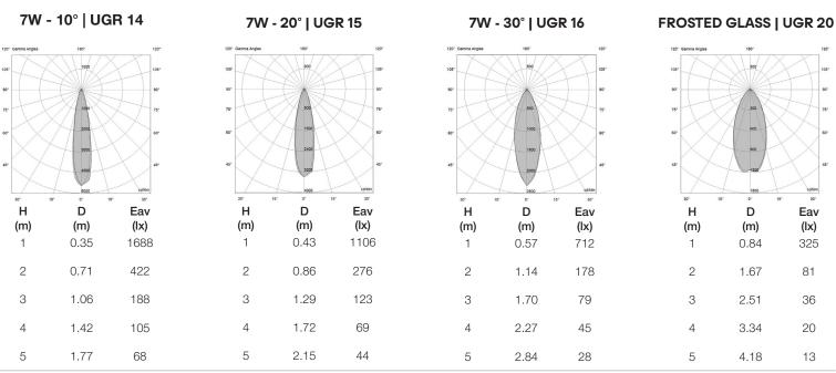
Total lumen output Total lumen output Total lumen output Total lumen output 565 lm 479 lm 519 lm 532 lm **Efficacy Efficacy** Efficacy **Efficacy** 83 lm/W 75 lm/W 79 lm/W 69 lm/W
