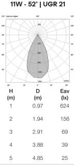
Total lumen output **Total lumen output** Total lumen output **Total lumen output** 857 lm 824 lm 809 lm 750 lm Efficacy Efficacy Efficacy Efficacy 78 lm/W 75 lm/W 74 lm/W 68 lm/W
